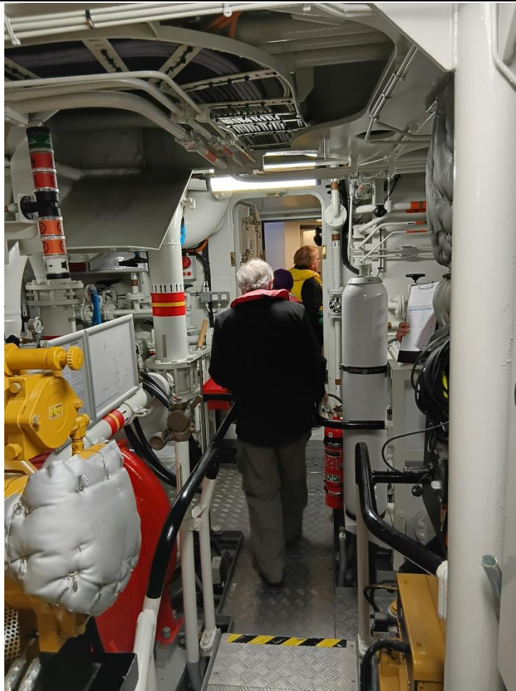
This is the two engine room with comparative walkways between the twin engines of both vessels. Top is Kaiana while below is twin locomotives engines started by compressed air. Kaiana has full flooding fire suppression system from the large compressed gas cylinders.
