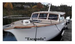
cover and table..... The entire deck has been covered with Teak, and front deck has been modified to receive a new winch and vents. New electrical includes, a third battery, new solar panel, new wiring and lights and auxiliaries include even blue underwater lighting .... About seven solid months of work on the hard at a local kiwi fruit farm. The original design was a 1947 Jim Young's pencil, built in 1949. The original size was 34' now extended to 38'.
