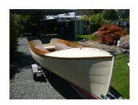
10. "Martha" Owned by Andy Hammond. A 14' Kauri clinker probably built by Seacraft - Auckland around 1950's. She has a 6hp single cylinder Petter diesel inboard engine. Martha now has a Mk.2 exhaust and a Mk.4 forward and reverse and is for sale.
