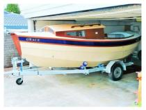
cockpit. Her name Grace, is a play on the design name "Tread Lightly" 2 ½ years to build in the shed. Carbon fibre 2 pce mast, 6hp 4 stroke outboard in motor well. Sleeps 2 comfortably. Full of BURNSCO accessories - from my work.
